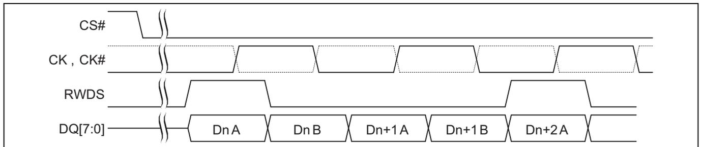
**Figure 8 Data placement during a write transaction<sup>[19-22]</sup>**
