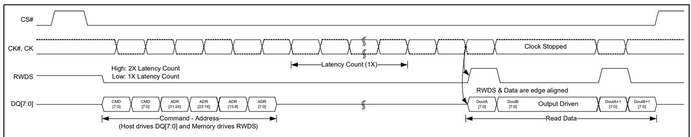
Figure 12 Active clock stop during read transaction (DDR)<sup>[46]</sup>
