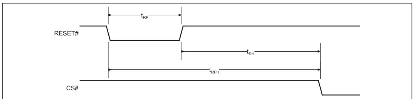
Figure 22 Hardware reset timing diagram
