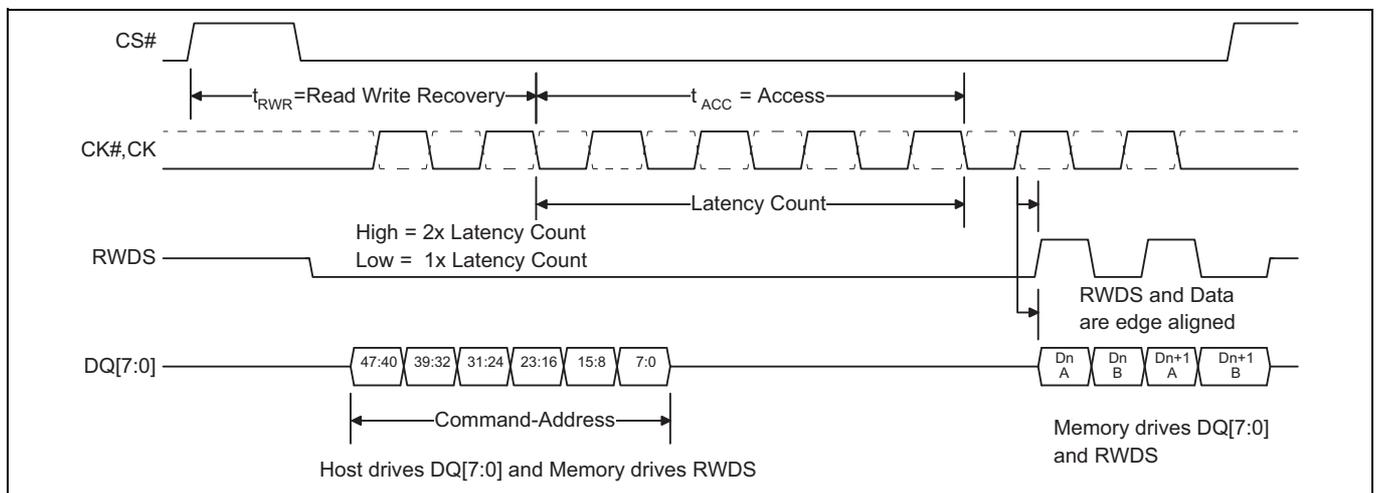
Figure 1 Read transaction, initial latency count<sup>[1]</sup>
