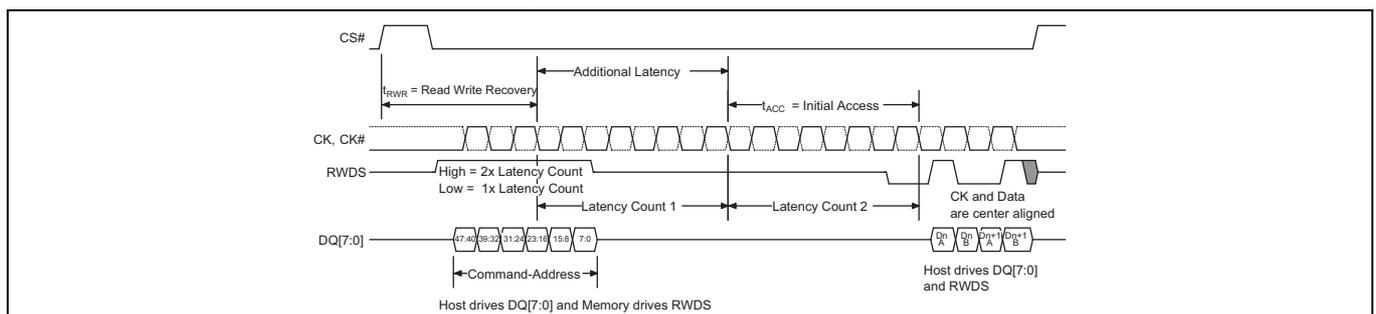
Figure 10 Write transaction with initial latency<sup>[32-38]</sup>
