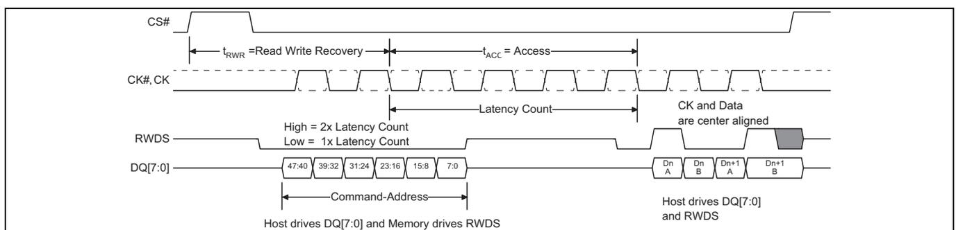
Figure 3 Write transaction, initial latency count<sup>[2]</sup>
