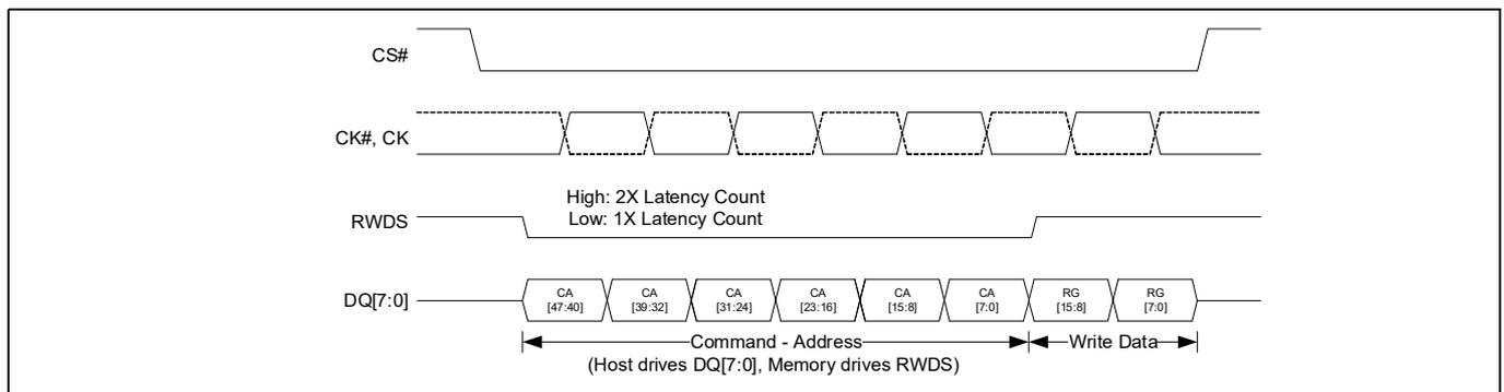
Figure 11 Register write operation<sup>[39, 40]</sup>
