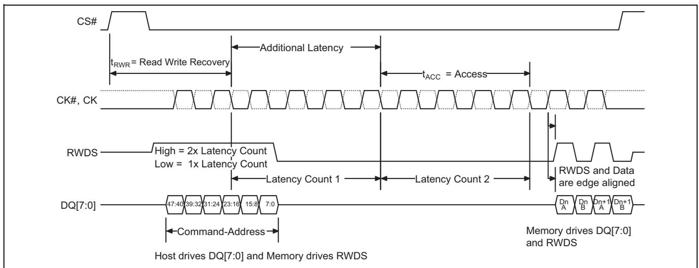
Figure 9 Read transaction with initial latency<sup>[23-31]</sup>
