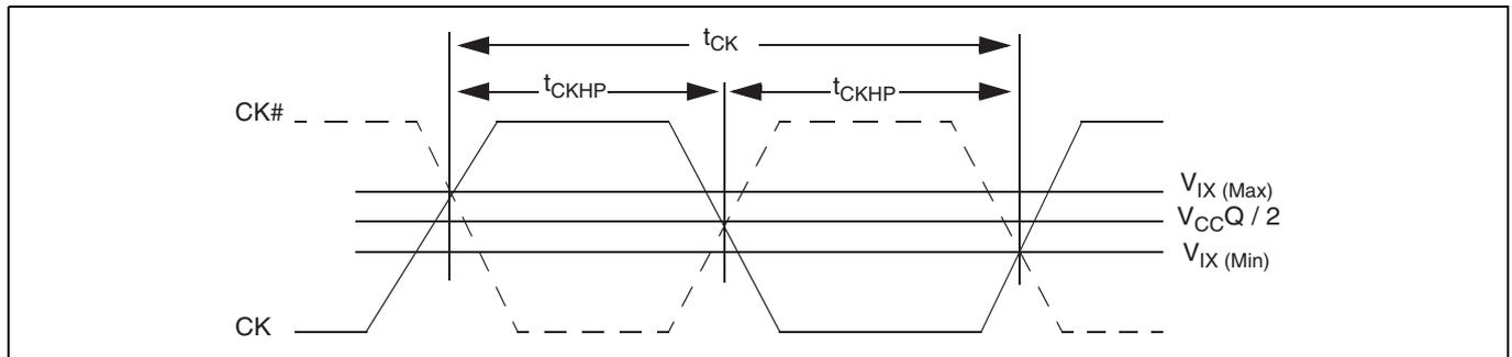
**Figure 26** Clock characteristics<sup>[65]</sup>
