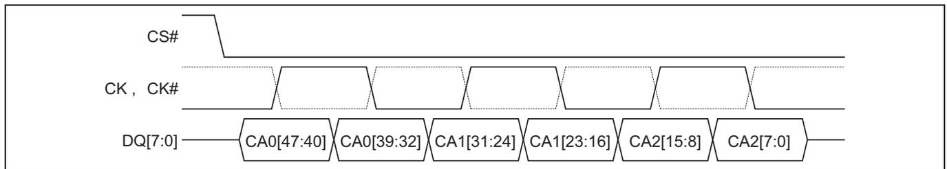
**Figure 6** Command-address (CA) sequence<sup>[6, 7, 8, 9]</sup>
