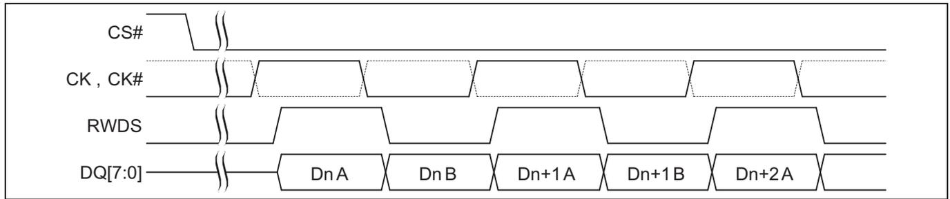
**Figure 7** Data placement during a read transaction<sup>[14-18]</sup>
