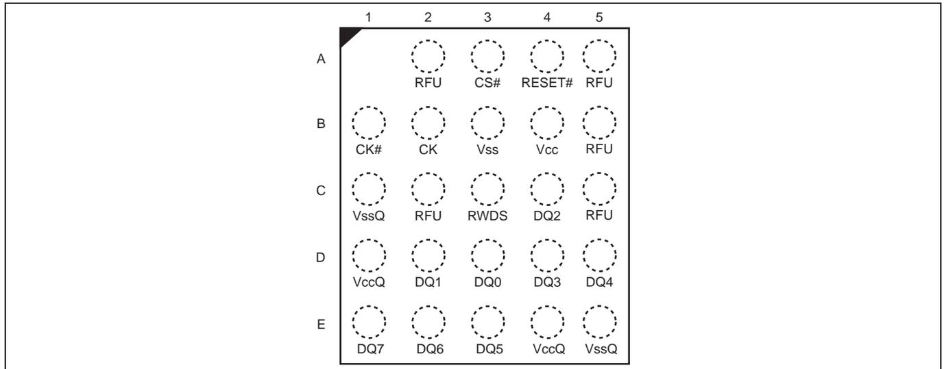
**Figure 33** 24-ball FBGA, 6 × 8 mm, 5 × 5 ball footprint, top view
