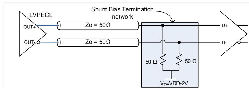
Figure 14. LVPECL with DC-coupled parallel shunt load termination
