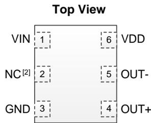
**Figure 4. Pin Assignments (3.2 x 2.5 mm package)**
