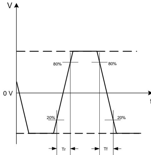
**Figure 8. LVDS Differential Waveform (i.e. OUT+ minus OUT-)**
