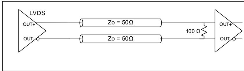
Figure 15. LVDS single DC termination at the load
