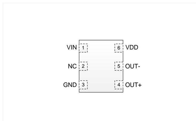
Figure 2. Pin Assignments (Top view)
