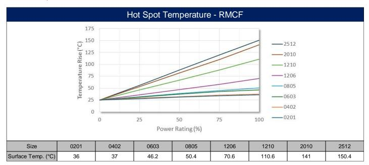
The thermal resistance of the RMCP will be similar to the RMCF. For example, the RMCF2512 and the RMCP2512 will have similar surface temperatures at 1W; the RMCP is designed to withstand higher temperatures associated with high power levels.
