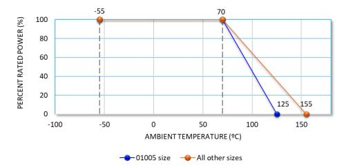
General Purpose Thick Film Standard Power and High-Power Chip Resistor
