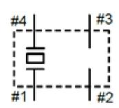
Pin #2 and #3 to be OPEN electrically to the PCB.
