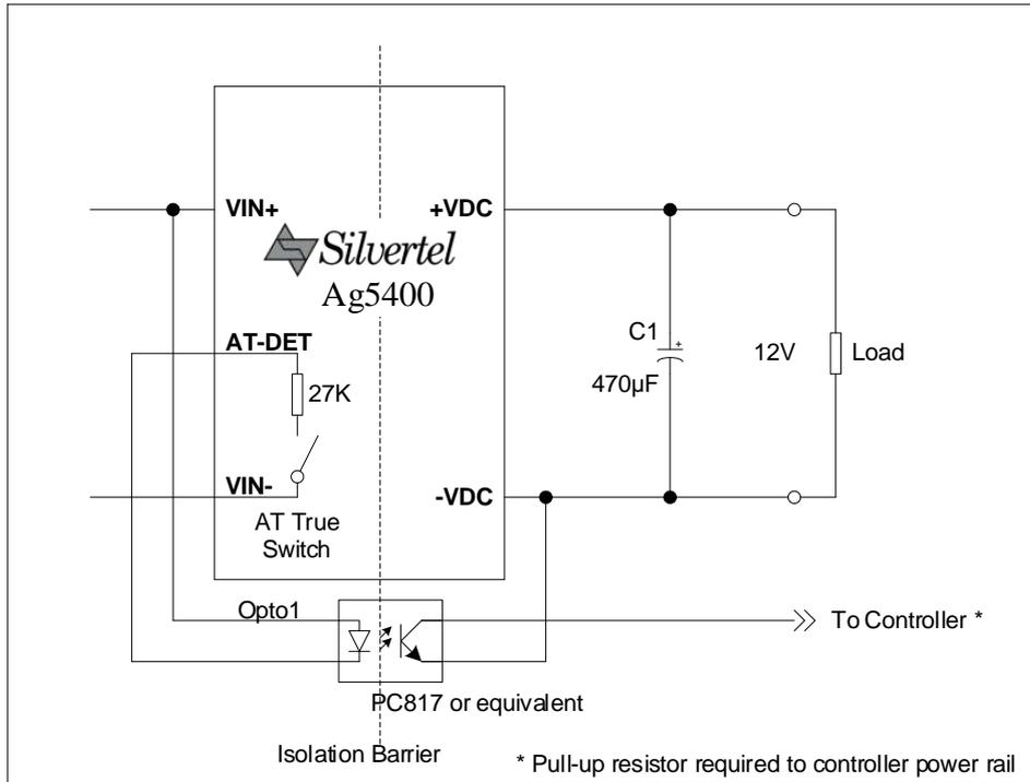
**Figure 4: Two Event Physical Layer Detect Configuration.**
