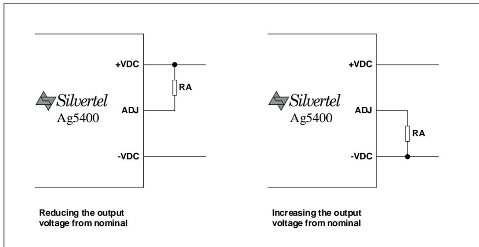
Figure 5: Output Voltage Adjustment
