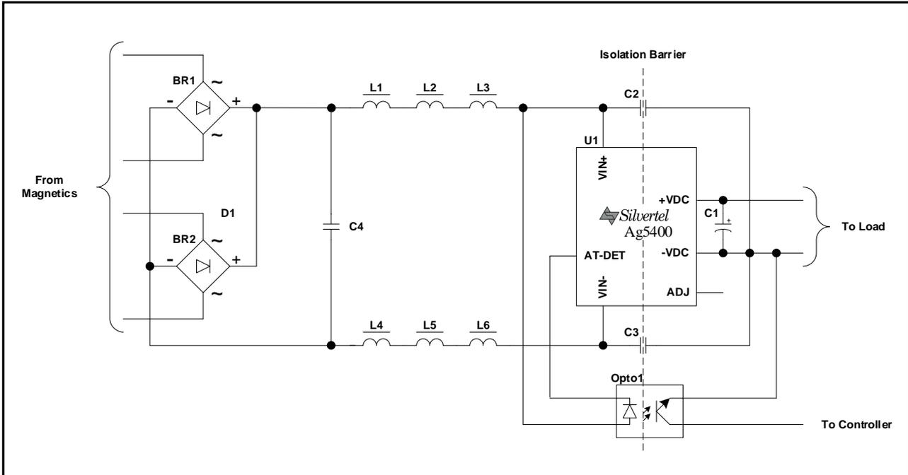
L1 – L6 = MPZ2012S102A, C1 = 470µF 16V, Opto1 = KPC357NT, C2 & C3 = 4.7nF 2000V, C4=10nF 100V,
