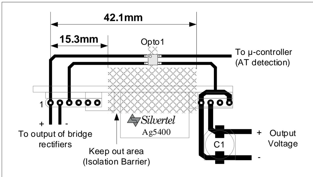
Figure 12: Isolation Barrier
