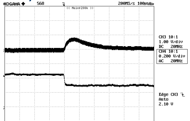
Figure 8: Output voltage response to step-change in load current (75%-50% of I_o , max; di/dt = 0.1A/\mu s ). Load cap: 10\mu F tantalum capacitor and 1\mu F ceramic capacitor. Top Trace: V_{out} (200mV/div, 100us/div), Bottom Trace: I_{out} (1A/div). Scope measurement should be made using a BNC cable (length shorter than 20 inches). Position the load between 51 mm to 76 mm (2 inches to 3 inches) from the module.
