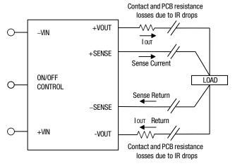
Figure 5. Remote Sense Circuit Configuration
