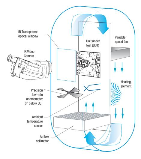
Figure 7. Vertical Wind Tunnel
