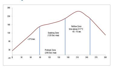
Optimal Peak 245°C, Max Peak 260°C. Lead-Free Solder type: SAC305
