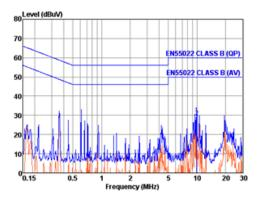
Graph 1. Conducted emissions performance, Positive Line, CISPR32, Class B, full load
