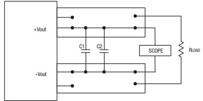
Figure 4. Measuring Output Ripple and Noise (PARD)
