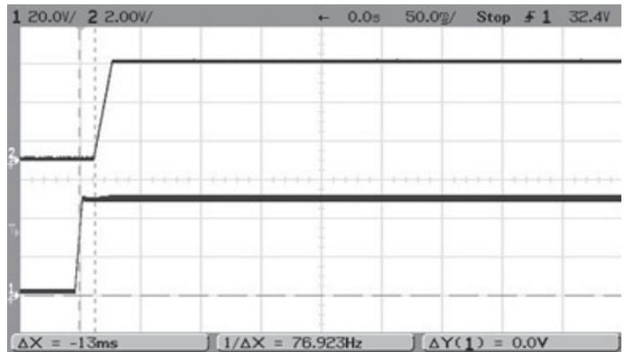
On/Off Enable Start-up (Vin = 48V, Vout = nom, Iout = 40A, Cload = 0, Ta = +25°C)
