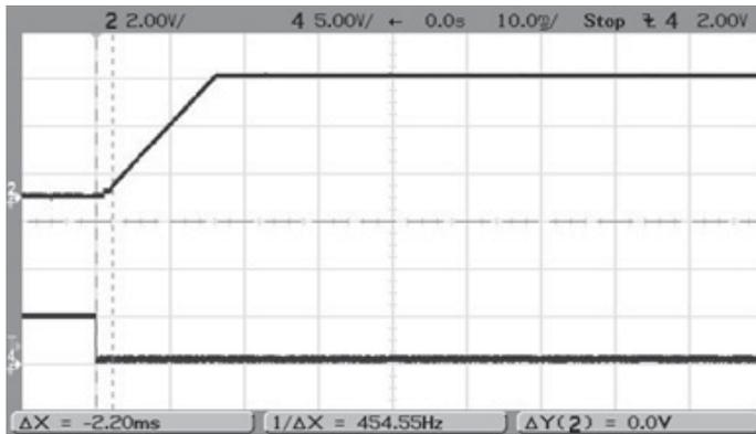
Start-up Delay (Vin = 48V, Vout = nom, Iout = 40A, Cload = 10000µf, Ta = +25°C)
