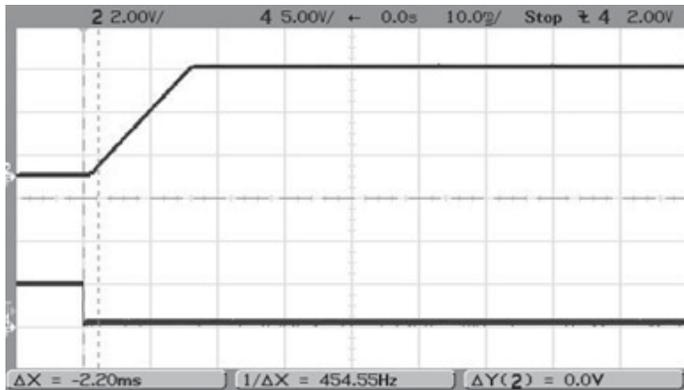
Start-up Delay (Vin = 48V, Vout = nom, Iout = 40A, Cload = 0, Ta = +25°C) ch1 = Vin,
