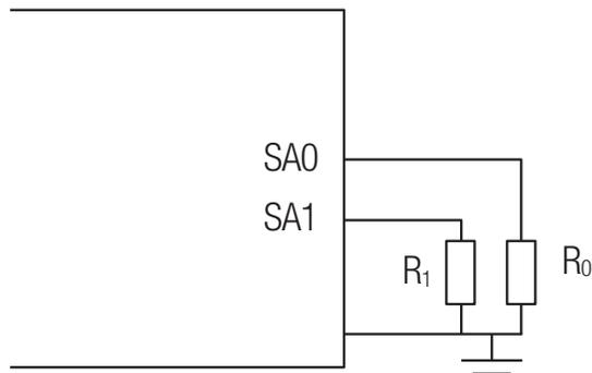
Figure 1. Schematic of Connection of Address Resistors
