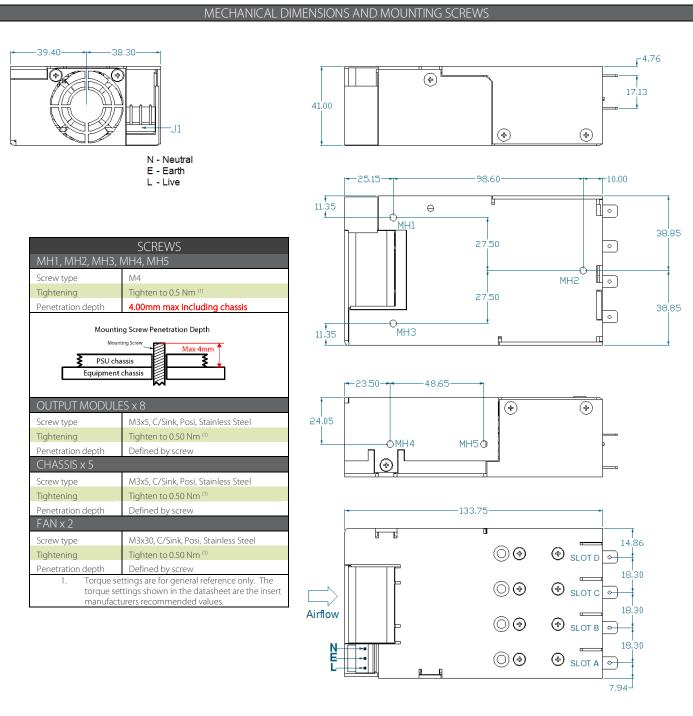
Airflow direction cannot be reversed
