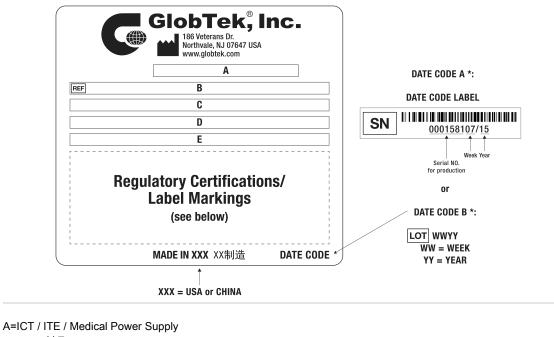
B=P/N: (料号) GTM962250P22533.5A-F C=Model (型号) GTM962250P22533.5A-F D=Input (输入)100-240V~, 50-60 Hz, 3A E=Output (输出)33.5 V == 6.71 A, 225.00 W
