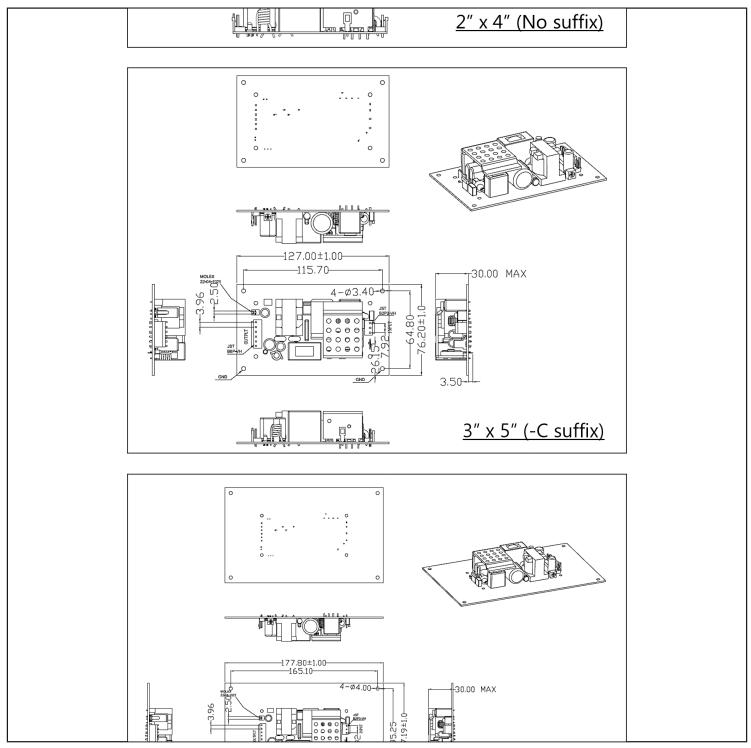
Drawing Title: GTM962250P22512A-F\_, ICT / ITE / Medical Power Supply, Efficiency Level: USA DOE Level VI / Eco-design Directive 2009/125/EC, (EU) 2019/1782, Case Color/Style: GlobTek Black, Open Frame/ L Frame/Cage/ Potted Internal, Regulated Switchmode AC-DC Power Supply AC Adaptor, Input Rating: 100-240V~, 50-60 Hz, PCB Pins, , Output Rating: 225.00W, 12.0V@17.55A, Pin Out: Pins 1, 2, 3: DC COM Pins 4, 5, 6: +V, Approvals:
