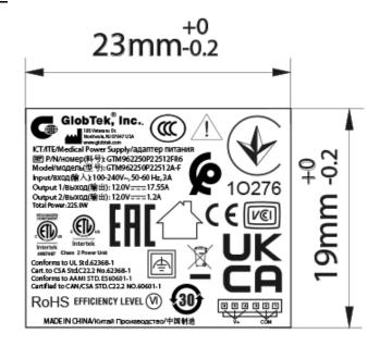
Drawing Title: GTM962250P22512A-F\_, ICT / ITE / Medical Power Supply, Efficiency Level: USA DOE Level VI / Eco-design Directive 2009/125/EC, (EU) 2019/1782, Case Color/Style: GlobTek Black, Open Frame/ L Frame/Cage/ Potted Internal, Regulated Switchmode AC-DC Power Supply AC Adaptor, Input Rating: 100-240V~, 50-60 Hz, PCB Pins, , Output Rating: 225.00W, 12.0V@17.55A, Pin Out: Pins 1, 2, 3: DC COM Pins 4, 5, 6: +V, Approvals:
