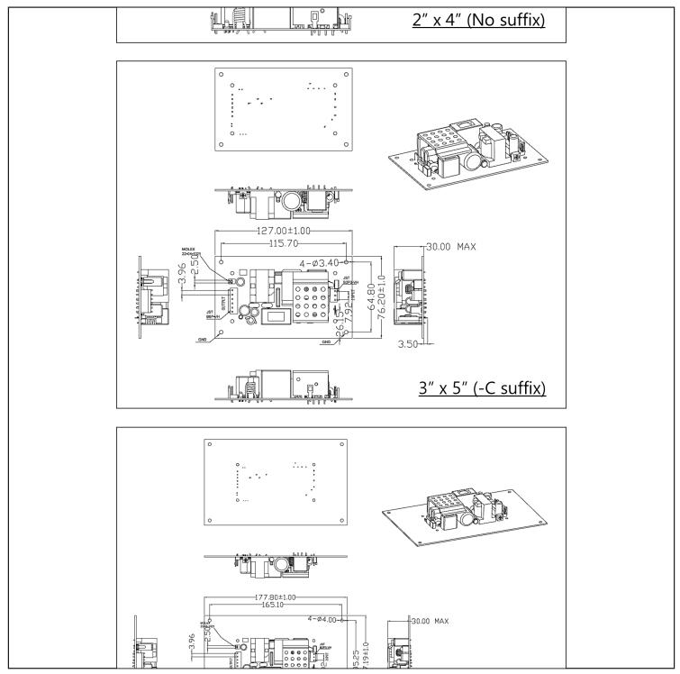
Drawing Title: GTM962250P22518A-F, ICT / ITE / Medical Power Supply, Efficiency Level: USA DOE Level VI / Eco-design Directive 2009/125/EC, (EU) 2019/1782, Case Color/Style: GlobTek Black, Open Frame/ L Frame/Cage/ Potted Internal, Regulated Switchmode AC-DC Power Supply AC Adaptor, Input Rating: 100-240V~, 50-60 Hz, PCB Pins, , Output Rating: 225.00W, 18.0V@12.5A, Pin Out: Pins 1, 2, 3: DC COM Pins 4, 5, 6: +V, Approvals:
