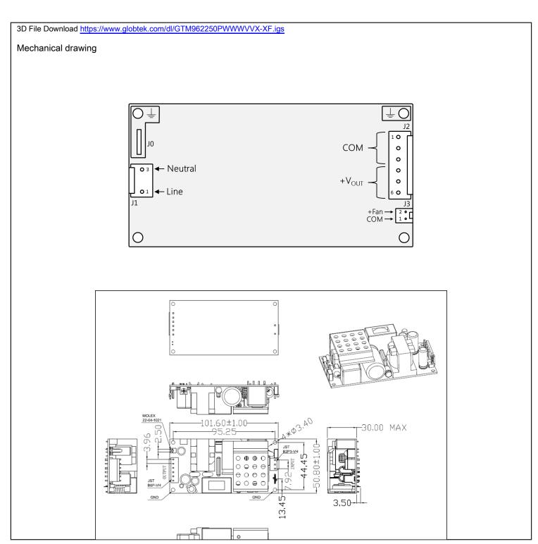
Drawing Title: GTM962250P22520A-F, ICT / ITE / Medical Power Supply, Efficiency Level: USA DOE Level VI / Eco-design Directive 2009/125/EC, (EU) 2019/1782, Case Color/Style: GlobTek Black, Open Frame/ L Frame/Cage/ Potted Internal, Regulated Switchmode AC-DC Power Supply AC Adaptor, Input Rating: 100-240V~, 50-60 Hz, PCB Pins, , Output Rating: 225.00W, 20.0V@11.25A, Pin Out: Pins 1, 2, 3: DC COM Pins 4, 5, 6: +V, Approvals:
