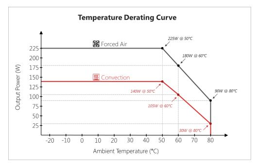
Drawing Title: GTM962250P22516A-F, ICT / ITE / Medical Power Supply, Efficiency Level: USA DOE Level VI / Eco-design Directive 2009/125/EC, (EU) 2019/1782, Case Color/Style: GlobTek Black, Open Frame/L Frame/Cage/ Potted Internal, Regulated Switchmode AC-DC Power Supply AC Adaptor, Input Rating: 100-240V~, 50-60 Hz, PCB Pins, , Output Rating: 225.00W, 16.0V@14.06A, Pin Out: Pins 1, 2, 3: DC COM Pins 4, 5, 6: +V, Approvals:
