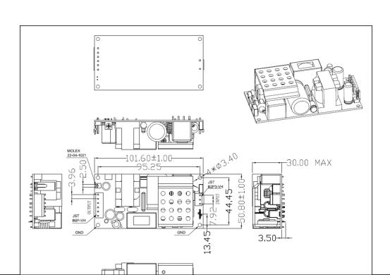
Drawing Title: GTM962250P22522A-F, ICT / ITE / Medical Power Supply, Efficiency Level: USA DOE Level VI / Eco-design Directive 2009/125/EC, (EU) 2019/1782, Case Color/Style: GlobTek Black, Open Frame/ L Frame/Cage/ Potted Internal, Regulated Switchmode AC-DC Power Supply AC Adaptor, Input Rating: 100-240V~, 50-60 Hz, PCB Pins, , Output Rating: 225.00W, 22.0V@10.22A, Pin Out: Pins 1, 2, 3: DC COM Pins 4, 5, 6: +V, Approvals:
