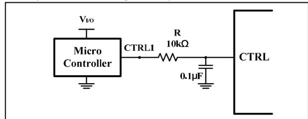
**Figure 19** AGC1 Mode Circuit
