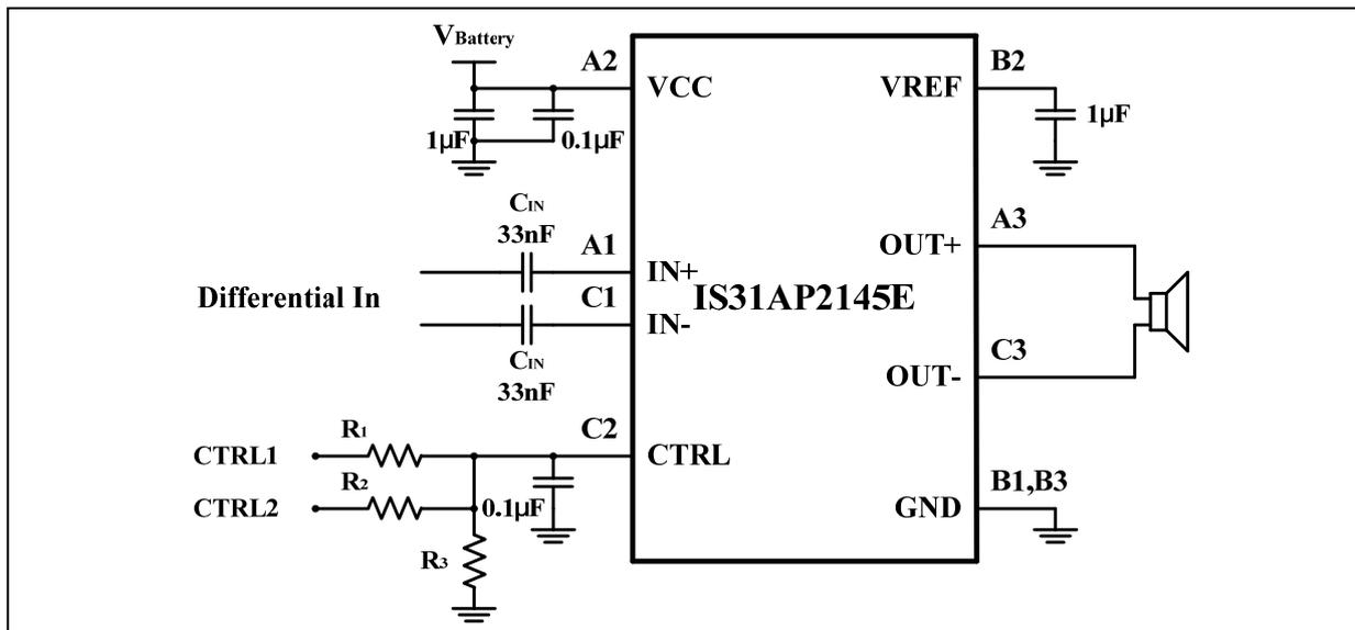
Figure 1 Typical Application Circuit (Differential Input)
