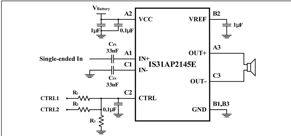
**Figure 2** Typical Application Circuit (Single-Ended Input)
