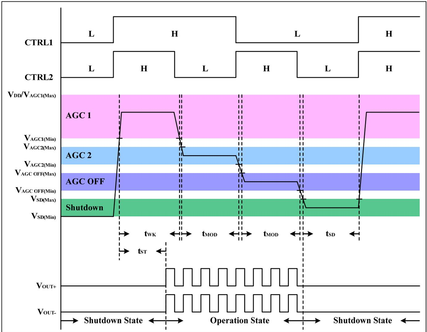
Figure 20 System Timing
