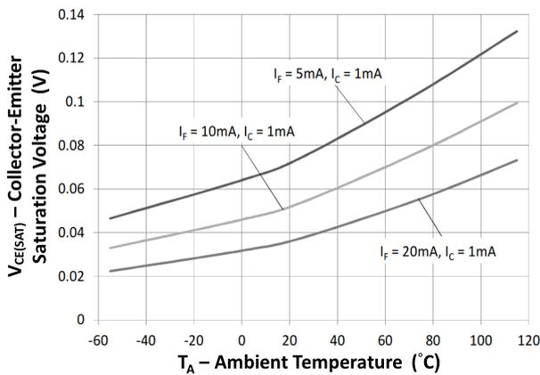
Fig 5 Collector-Emitter Saturation Voltage vs Ambient Temperature
