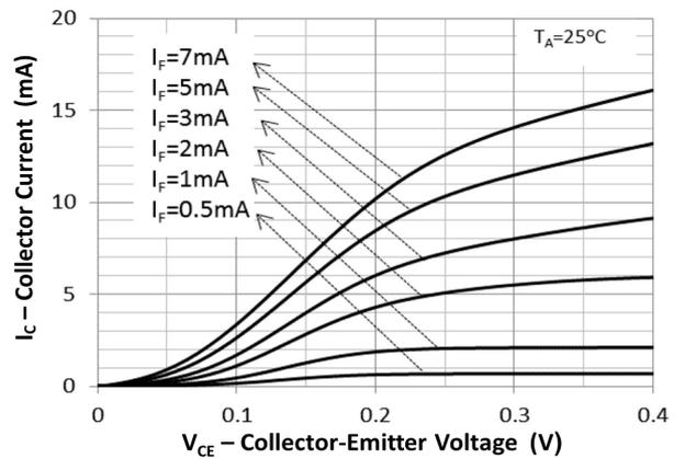
Fig 4 Collector Current vs Collector-Emitter Saturation Voltage
