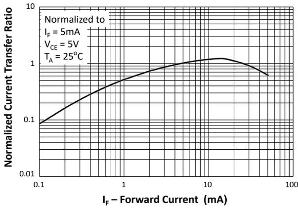
Fig 7 Normalized Current Transfer Ratio vs Forward Current
