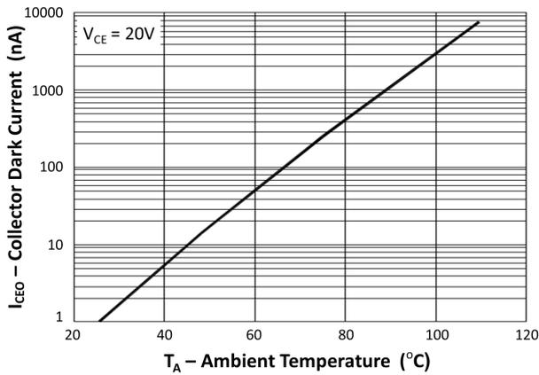
Fig 9 Collector Dark Current vs Ambient Temperature
