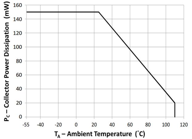
Fig 2 Collector Power Dissipation vs Ambient Temperature
