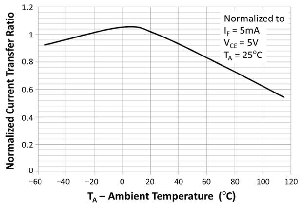
Fig 8 Normalized Current Transfer Ratio vs Ambient Temperature
