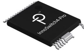
Figure 2a. High Creepage, Safety-Compliant InSOP-T28D Package.
