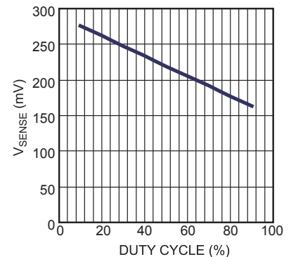
Figure 2: V_{SENSE} vs Duty Cycle
