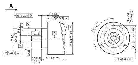
General tolerances according to DIN ISO 2768-mk ① Cable diameter = 5.6 mm + /-0.2 mm bend radius = 30 mm
