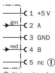
Voltage supply connection diagram
