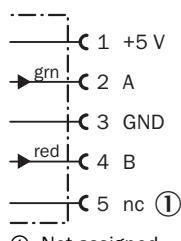
Voltage supply connection diagram
