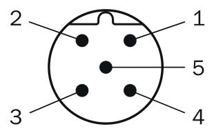
Connector M12, 5-pin, A-coded
