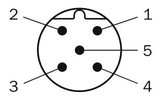
Male connector M12, 5-pin, A-coded
