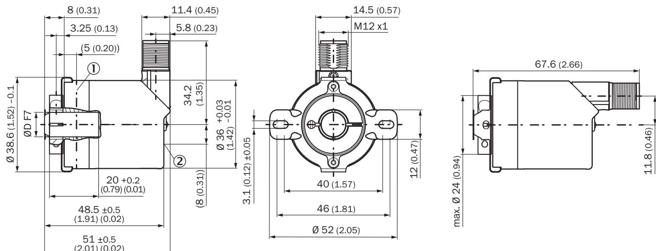
① Measuring point for operating temperature
