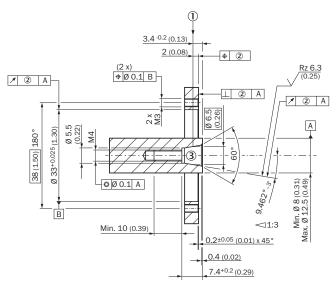
Read out axial position: positive value shows movement of rotor away from the motor flange; negative value shows movement of rotor towards the motor flange
