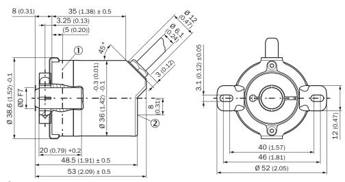
$\textcircled{\sc 0}$  Measuring point for operating temperature
