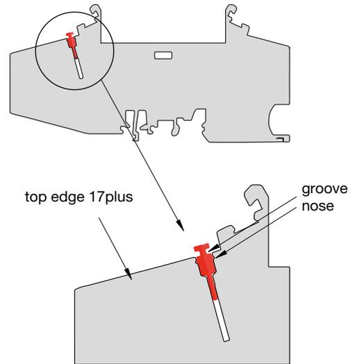
When mounting several modules side by side, proper insertion of the 32 A busbar X 222 005 01/02/03 has to be observed, i.e. the busbar must be pushed in evenly across the whole length from left to right, repeatedly if necessary. The groove of the busbar must be flush with the top edge of the Module 17plus.
