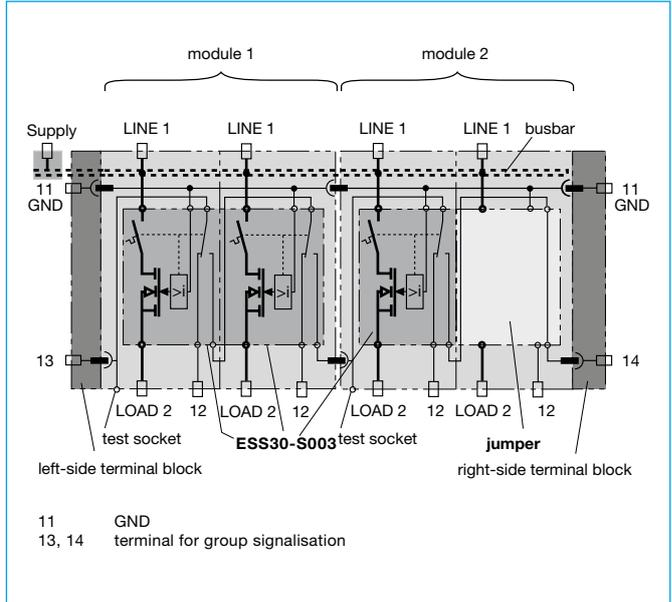
**Pin selection, fitted with ESS30-S003**
