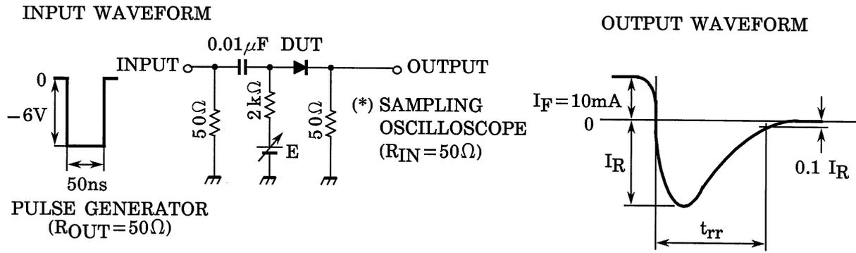
Fig.1 Reverse Recovery Time (t<sub>rr</sub>) Test Circuit
