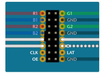
Pins A, B, C and D select which two rows of the display are currently lit. (32x16 matrices don't have a "D" pin — it's connected to ground instead.)
