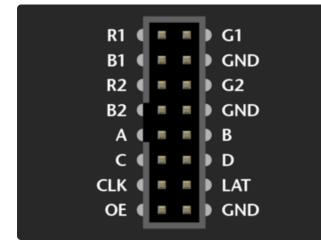
The layout is very similar to the 32x16 panel, with pin "D" replacing one ground connection.
