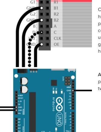
Current **Arduino Uno form-factor** boards have **three** ground pins (the third is next to pin 13). If you need additional ground connections — for a 32x16 matrix, or if using an older Arduino board with only 2 ground pins — a solderless breadboard is handy for linking all these pins.
