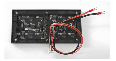
If your power cable came with spades at the opposite end of this power cable, they can be screwed into a 2.1mm terminal block adapter. Works nicely! Don't allow the exposed connectors to contact metal though...you should probably cover this with heat-shrink tube or electrical tape.
