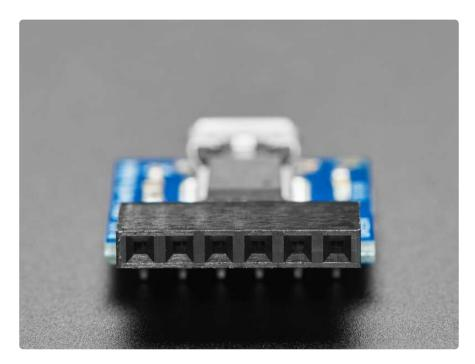
By default, we've set it up so that it matches our FTDI cables. The 6th pin is RTS (as of Arduino IDE v1.8 this will work perfectly for uploading to 'inos), the power wire is +5V and the signal levels are 3.3V (they are 5V compliant, and should work in the vast majority of 3.3V and 5V signal systems).
