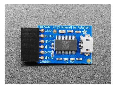
Long gone are the days of parallel ports and serial ports. Now the USB port reigns supreme! But USB is hard, and you just want to transfer your every-day serial data from a microcontroller to computer. What now? Enter the FTDI Friend!
