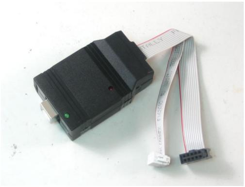
There are two ways to program an AVR microcontroller. One is to reprogram the entire chip using an AVR programmer. The other is to use a **bootloader** that is preprogrammed onto the chip that allows the chip to re-program itself. An AVR programmer is more powerful: you can really mess with anything on the chip and the entire 32K of memory is available. Using the bootloader is safer: there's no way to mess with the fuse settings (which could brick the chip) but you only get 30K of
