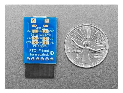
The FTDI Friend is a tweaked out FTDI FT232RL chip adapter. Sure, like the well-known FTDI cable, it can provide power to your project and there are 4 signal lines for sending data back and forth. But the Friend can do much more! For example, you can change the signal and power lines to be either 3.3V or 5V. Arduino-derivatives and
