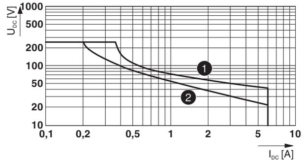
Figure 6 Relay load curve - ohmic and inductive load
