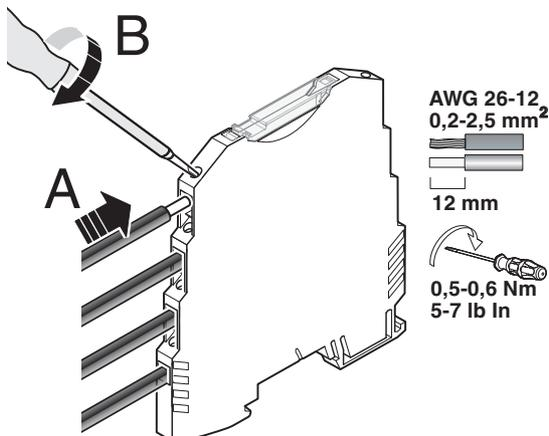
Figure 9 Connection of the cables
