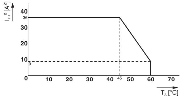
Figure 5 Derating curve - vertical or horizontal mounting position, without spacing
