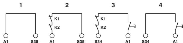
Figure 11 Start and feedback circuit connection variants
