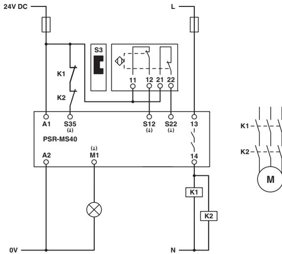
Figure 14 Magnetic switch monitoring/automatic start
