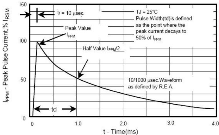
Fig.3 - Pulse Waveform
