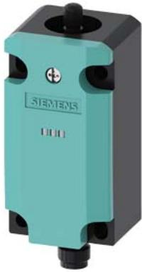
Basic switch for position switch 3SE51 Metal enclosure 40 mm according to EN 50041 1 NO/1 NC slow-action contacts with M12 connector, 5-pole, fixed with 2 LEDs, yellow/green, 24 V DC without actuator head Pin assignment: Pin1=21, Pin2=22 Pin3=14 and LED green, Pin4=13 and LED yellow, Pin5=ground LED
