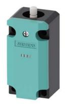
Basic switch for position switch 3SE51 Plastic enclosure 40 mm according to EN 50041 Device connection 1 x (M20 x 1.5) with 2 LEDs, yellow/green, 24 V DC 1 NO/2 NC slow-action contacts without actuator head
