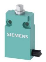
Position switch in compact design 30 mm wide with connecting cable 5 m Snapaction contacts 1 NO+1 NC with rounded plunger
