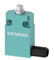
Position switch in compact design 30 mm wide with connector plug M12 Snapaction contacts 1 NO+1 NC with rounded plunger
