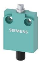
Position switch in compact design 40 mm wide with connector plug M12 Snapaction contacts 1 NO+1 NC with rounded plunger
