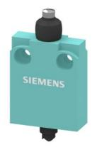
Position switch in compact design 40 mm wide with connection cable 2 m Snapaction contacts 1 NO+1 NC with rounded plunger with exterior seal
