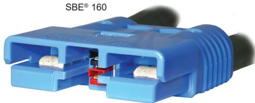
SBX® and SBE® connectors can integrate up to 8 auxiliary power / signal contacts along with the two primary power circuits. SBE® connectors feature an IEC 60950 touch safe housing molded from a chemical resistant PBT / PC blend resin. SBX® are molded from a rugged PC resin and are rated IP20 per IEC 60529.
