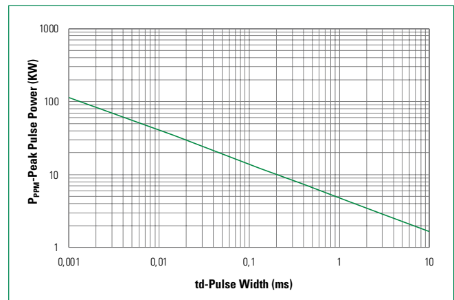
Figure 2: Peak Pulse Power Rating
