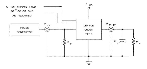
minimum or equivalent (includes test jig and probe capacitance).
