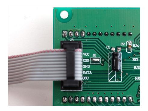
You should also check that the **J5** solder jumper is 'filled' with solder - you need to have **J5** shorted for using one or two panels in a cascade. Use a soldering iron to heat up some solder and melt it on to **J5** if it isn't filled yet.
