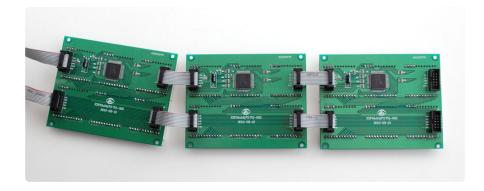
Finally, you will need to use both IDC cables. The first (top left) cable has **VCC** and **GND**, as well as **DATA** and **WRITE** as in the previous tests.
