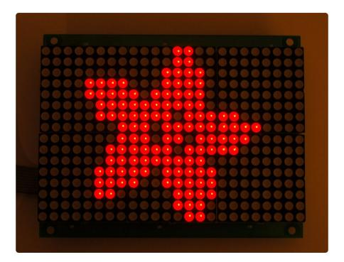
These LED panels take care of all the work of making a big matrix display. Each panel has six 8x8 red matrix modules, for a 16x24 matrix. The panel has a **HT1632C** chip on the back with does all the multiplexing work for you and has a 3-pin SPI-like serial interface to talk to it and set LEDs on or off. There's a few extras as well, such as being able to change the brightness of the entire display, or blink the entire display at 1 Hz.
