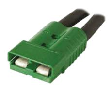
The SB\* 350 is the largest connector in the series with power capabilities up to 500 amps with a 350 mcm wire. Wires ranging from 1/0 to 350 mcm (53.5 to 185 mm²) fit into the one piece housing available in standard PC or a chemical resistant PBT/PC blend. Silver plated wire or busbar contacts minimize electrical resistance while offering supreme durability and reliability.
