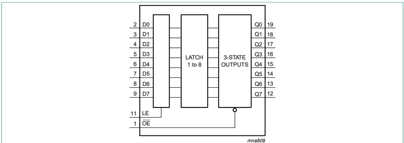
Fig. 1. Functional diagram
