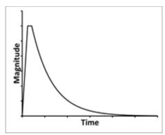
The electrochemical sensor output has the normal power-on startup profile pictured here.
