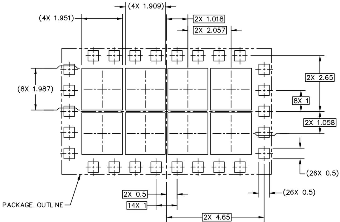
PCB DESIGN GUIDELINES – SOLDER MASK OPENING PATTERN
