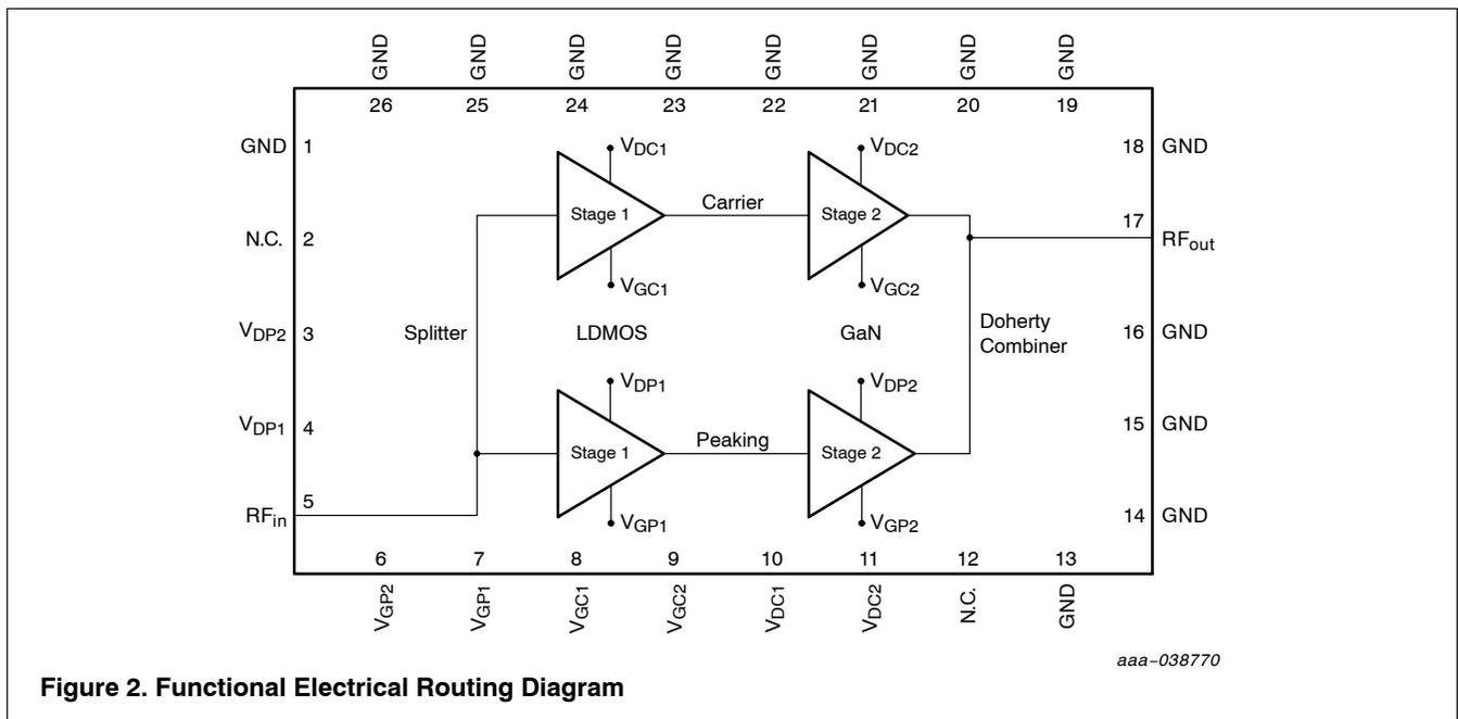
**Figure 2. Functional Electrical Routing Diagram**
