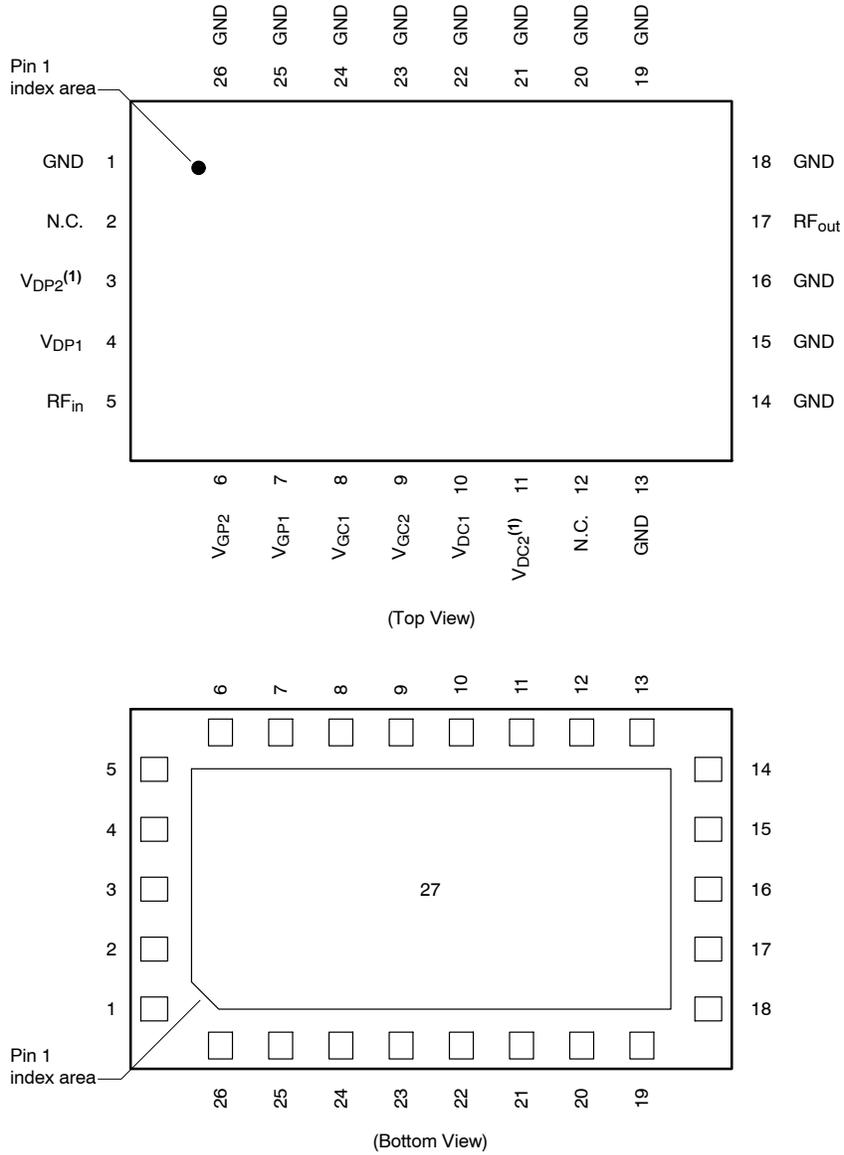
**Figure 1. Pin Connections**
