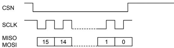
**Figure 25: 16-Bit SPI Frame**
