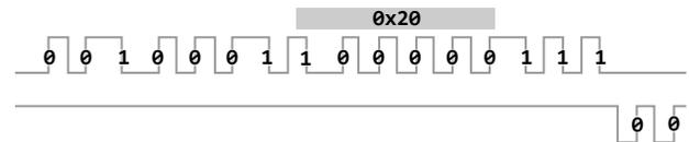
**Figure 34: Target ID = [0 0 0 1], ANGLE = 0x20, CRC = 111**
