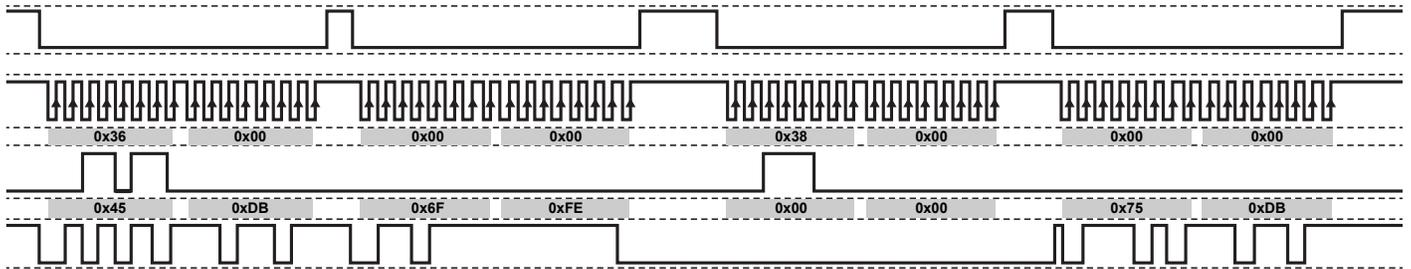
Figure 18: Read of a Negative TURNS\_DELTA Value
