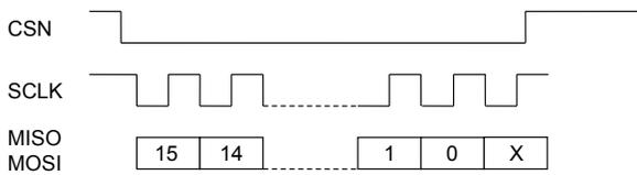
**Figure 26: 17-Bit SPI Frame**
