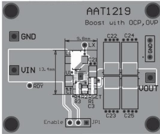
**Figure 3: AAT1219 Evaluation Board Top Side Layout.**
