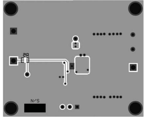
**Figure 4: AAT1219 Evaluation Board Bottom Side Layout**
