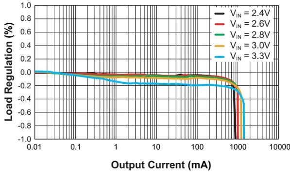
**Load Regulation vs. Output Current**
