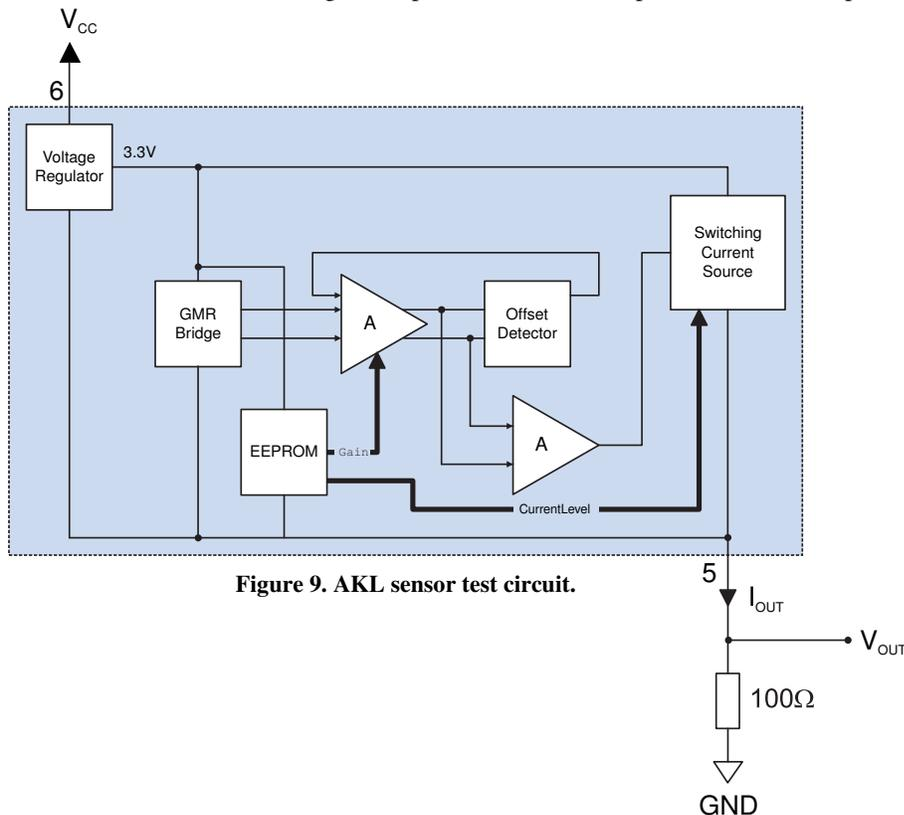
Figure 9. AKL sensor test circuit.
