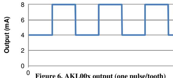
**Figure 6. AKL00x output (one pulse/tooth)**
