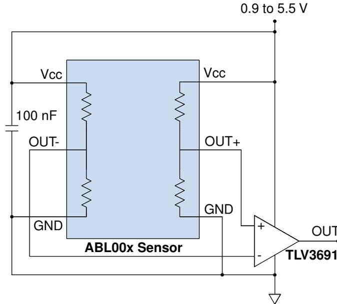
**Figure 7. Digital output from an analog sensor.**
