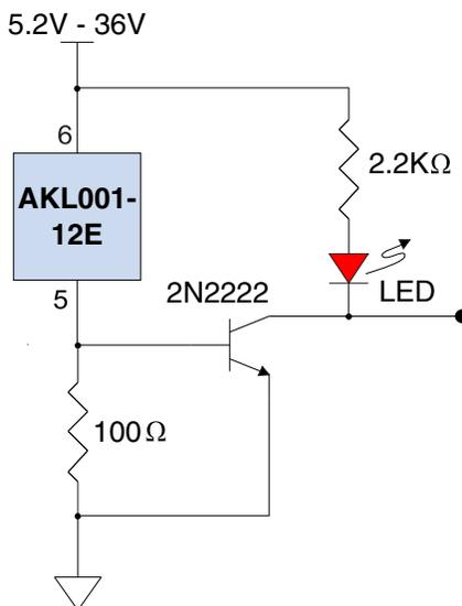
Figure 10. Simple three-wire interface.
